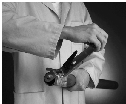
Chamfering the pipe
