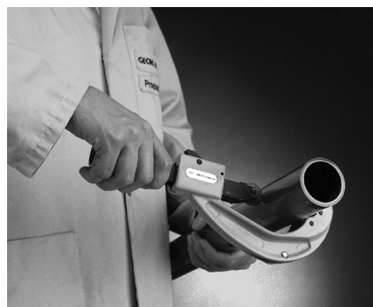
Cutting the pipe to length
